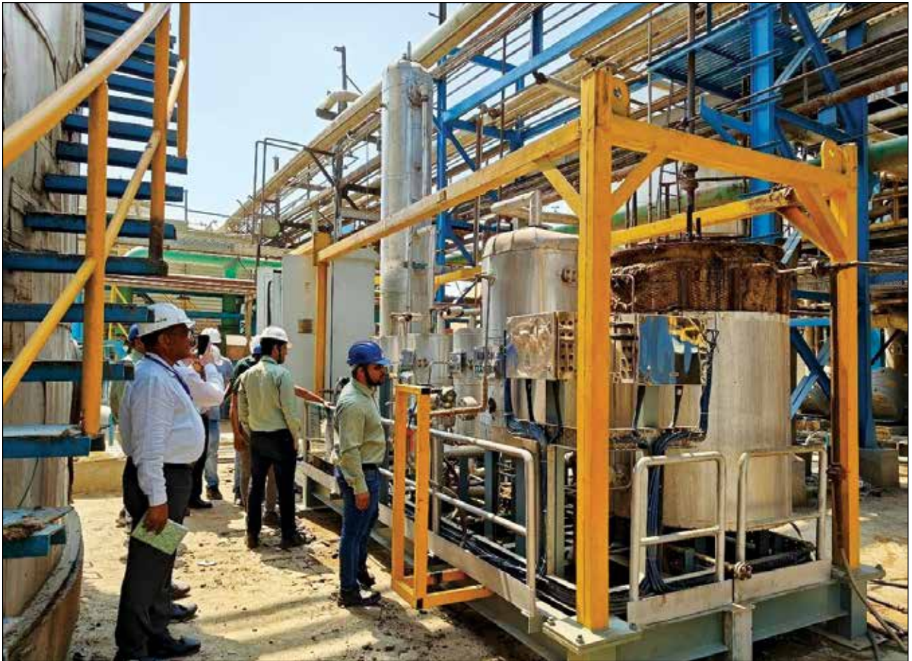
Transportable pilot demonstration unit for black liquor heat treatment technology under paper (phase 2) project
