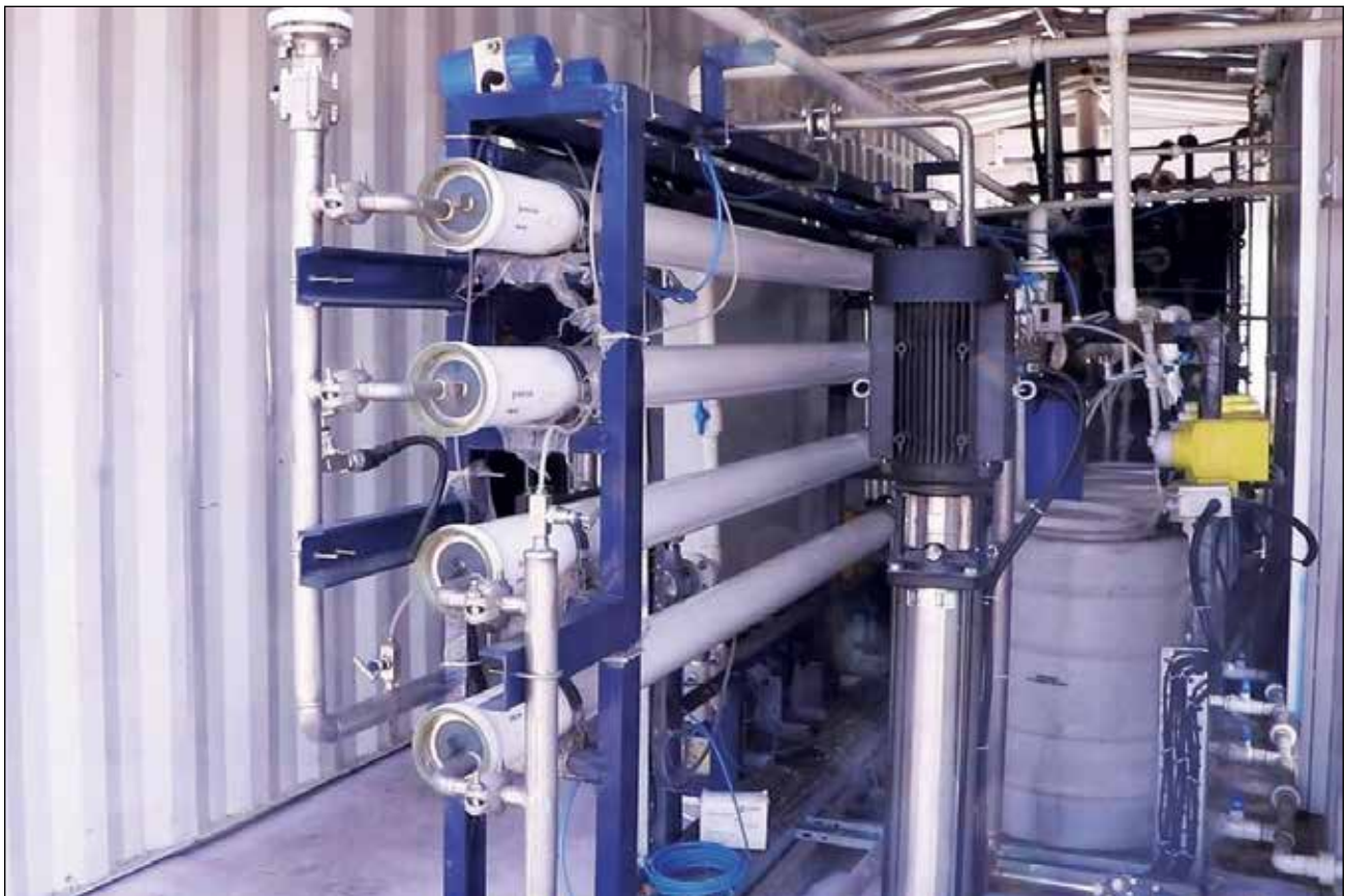
Containerized pilot demonstration unit for membrane filtration technology under paper (phase 2) project
